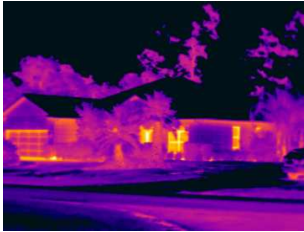
Description: IR Image #13 Thermal image of ICF construction
